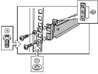
Figure 37: Attaching Rail Brackets to Post
